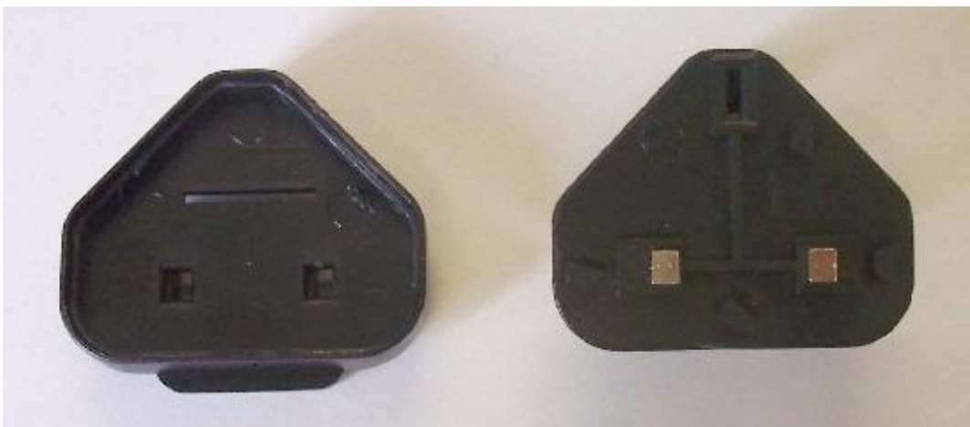
The failed/detached plug plate
